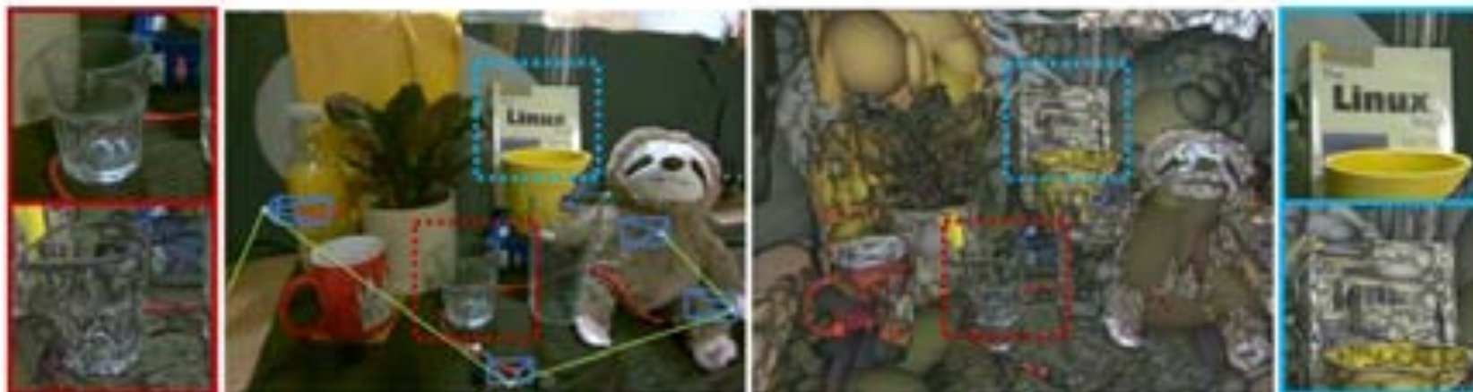
Figure 1. From a single monocular camera, we reconstruct a high fidelity 3D scene live at 30fps. For every incoming RGB frame, 3D Gaussians are incrementally formed and optimised together with the camera poses. We show both the rasterised Gaussians (left) and Gaussians shaded to highlight the geometry (right). Notice the details and the complex material properties (e.g. transparency) captured. Thin structures such as wires are accurately represented by numerous small, elongated Gaussians, and transparent objects are effectively represented by placing the Gaussians along the rim. Our system significantly advances the fidelity a live monocular SLAM system can capture.
