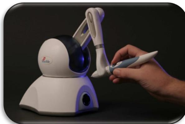
Figure 4 - SensAble's Phantom Omni Haptic Device
