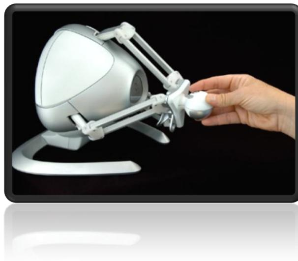
NOVINT® provides an SDK API which can be used using C++. The API is divided in three layers: DHDLC (low-level drivers), HDAL (mid-level device communication) and Falcon API (high-level programming toolset).
