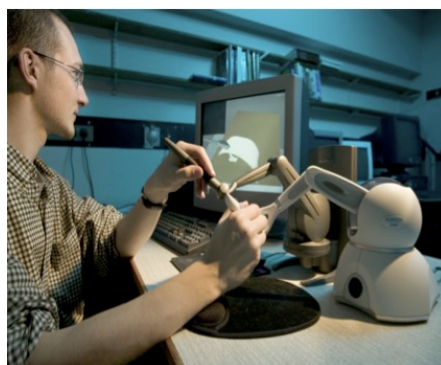
Figure 1.9: Two Haptic devices are used to simulate the needle puncture (Phantom)
