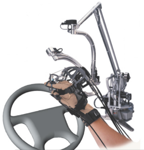
Figure 1.5: The Haptic armature gives the user the feeling of manipulating a wheel
