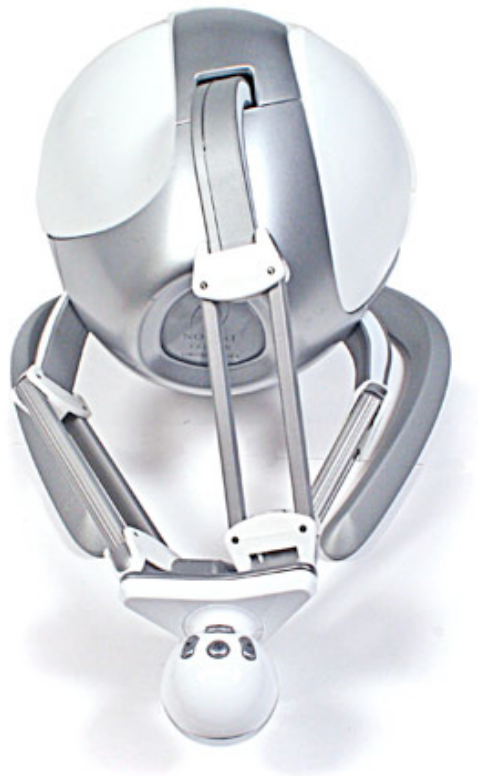
Figure H : Picture of the Novint Falcon haptic device. We can see the handgrip in the foreground held by three mobile arms coming from the main body. [47]
