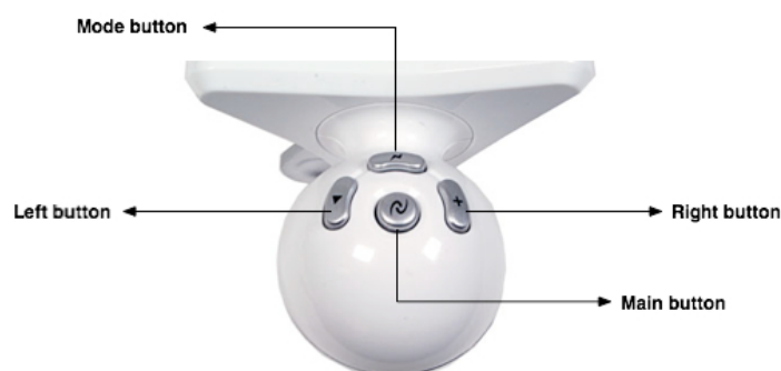
Figure N : Controller of the Falcon Novint haptic device
