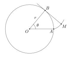
Figure 4: The construction of an involute.
