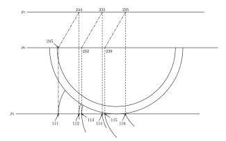
**Figure 9**: Step 2. Involutes tangent to the vertical lines going through  $z_{111}, \ldots, z_{116}$ .
