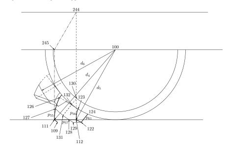
Figure 11: Step 3. Construction of the upper teeth: the lines (123,126) and (112,111) are two of the generating lines of the surface making up the helical teeth.
