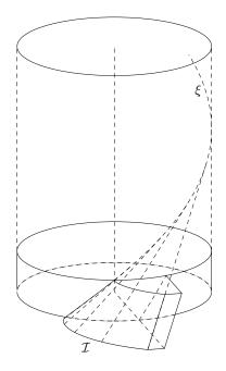
**Figure 6**: Helical tooth with involute profiles. The tooth is generated by an involute  $\mathcal{I}$  moving along a helix  $\xi$ . (In this drawing, the four non-working faces of the tooth have been made planar.)
