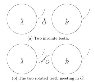
Figure 5: The contact of two involute teeth.
