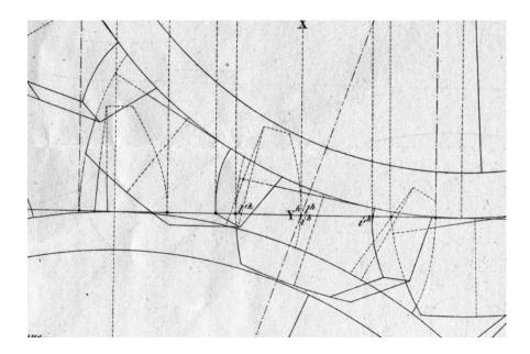
Figure 10: Excerpt of Olivier's plate: upper teeth construction.
