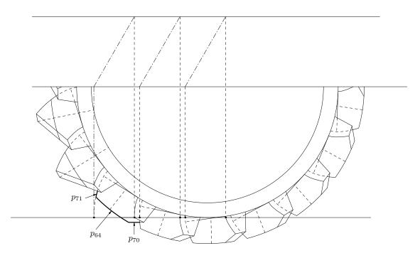
Figure 12: Step 4. Construction of the upper wheel contour.
