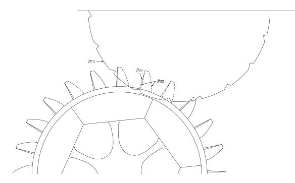
Figure 13: Step 5. Lower wheel teeth construction, and dashing.
