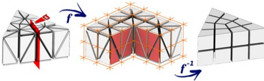
Figure 2: Global parameterization example: the input is cut open along the red plane (left), then it is deformed (middle), and the pre-image of the orange grid produces a hexahedral mesh (right).
