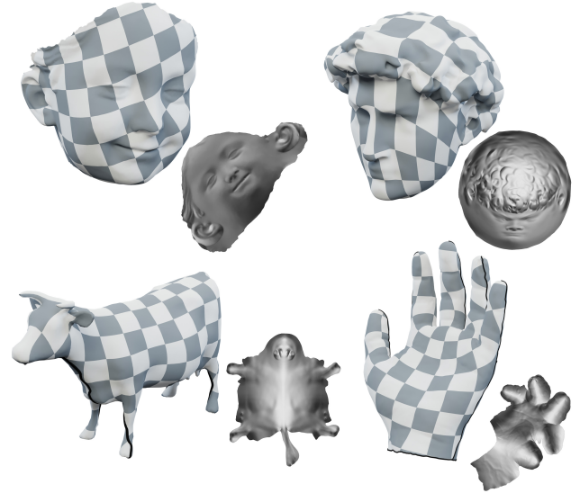
Fig. 17. Free boundary parametrization using our algorithm on disk-shaped models (top), or models with user-prescribed seams (bottom).
