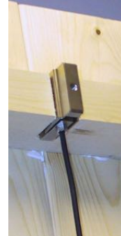
(b) An enlarged view of the load cell supporting the floor.
