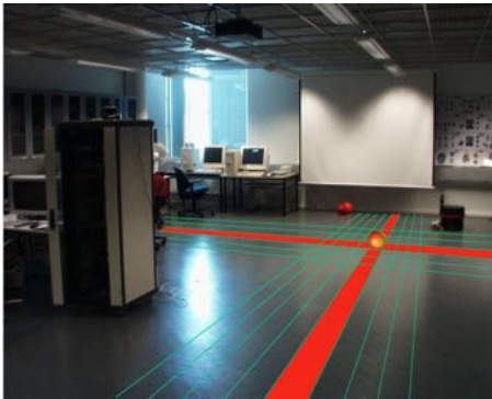
Figure 2.9 – The sensing floor composed of EMFi stripes, presented by Pirttikangas et al. in [110].
