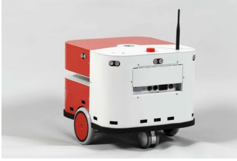
(a) A nonholonomic robuLAB-10 robot by RoboSoft, used in our experiment, weighing 35.7 kg. Source: www.robosoft.com
