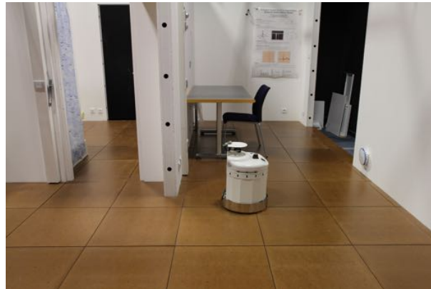
Figure 3.4 – PeKeeII robot communicating with an interactive sensing floor
