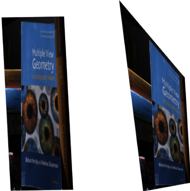
Fig. 4. A simulation example. These simulated views correspond to a view of the book cover which would be obtained from the camera whose pose is sought (in cyan in Figure 1), simulated from the far right real image. On the left: simulation with an affine transformation. On the right: simulation with a homography. Up to a slight rotation, the homography simulation of the cover is more like the actual view (in Figure 2 a).
