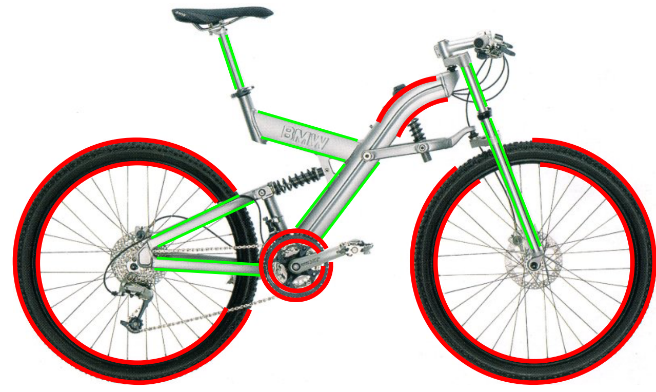
Fig 1: Arc and segment detection of an image
