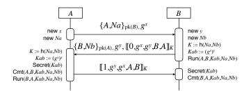
Figure 5. Key agreement protocol using asymmetric encryption (sk3<sub>asym</sub>)
