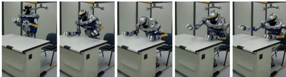
Figure 11. Screenshots captured from the sitting real world experiment using an open-loop full-motion optimization method.
