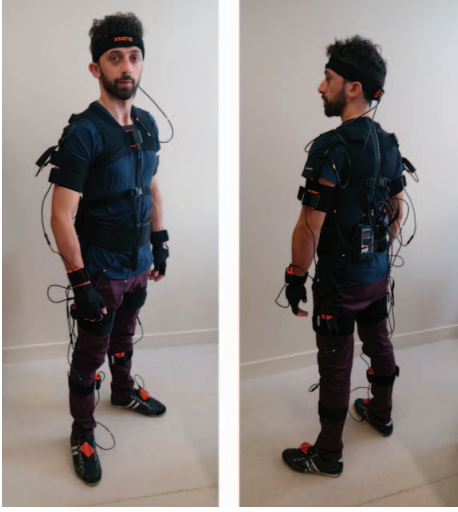
Fig. 1: Front and rear view of the human subject wearing the Xsens system
