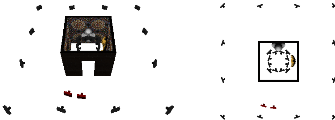
Fig. 10: Cameras for the building scene. Cameras were placed in both the interior and exterior of a building to enable simultaneous, complete reconstruction of its exterior and interior surfaces. The viewpoints used by the carving algorithm are shown in gray; the two red cameras correspond to the building’s views in Figs. 12(a)-(d).
