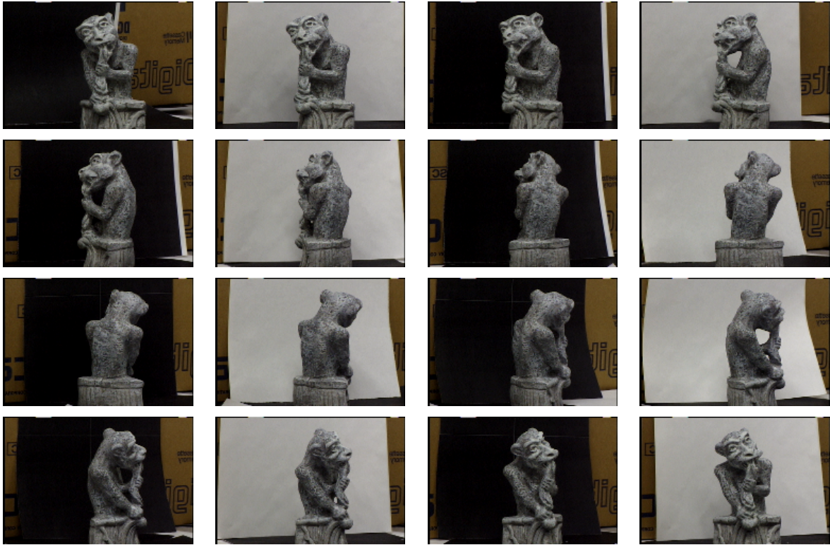
Fig. 8: A sequence of sixteen 486x720 RGB images of a gargoyle stone sculpture. The sequence corresponds to a complete rotation of the object in front of a stationary camera, performed in 22.5 degree increments.
