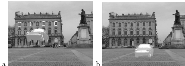
Fig. 5. (a) Registration using only 2D/3D correspondences. (b) Registration with the mixing method.
