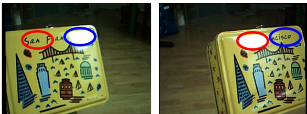
Figure 5.1 - Example of specular surfaces problem
