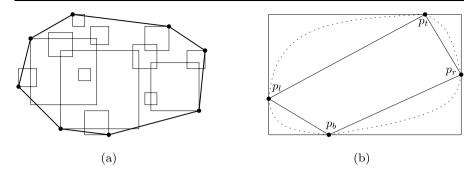
Fig. 6 (a) The largest area convex hull for a set of squares. (b) The four extreme points
