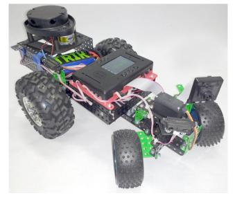
Fig. 7 Car with lidar and camera
