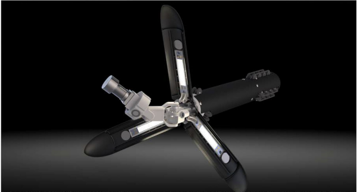
Image 2 : 3D rendering of the imaging robot with the pan-tilt camera (open) (artist view)
