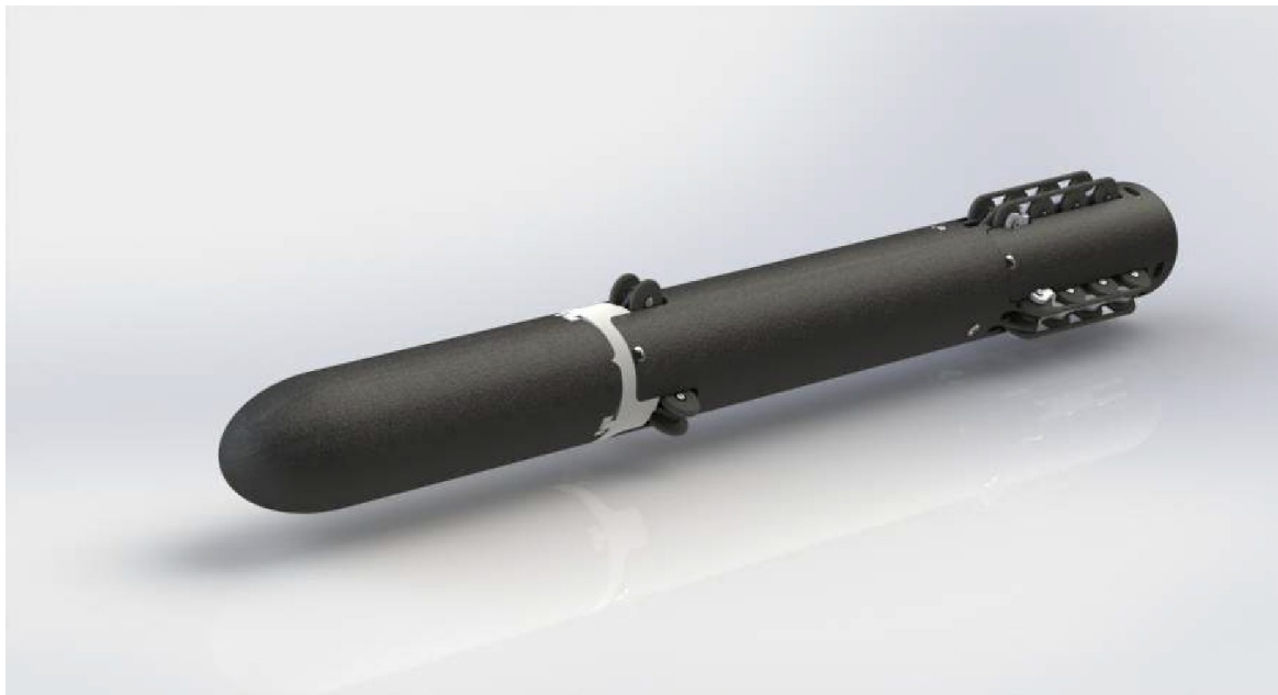
Image 4 : 3D rendering of the imaging robot with the pan-tilt camera (closed) (artist view)
