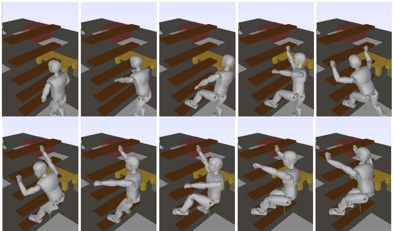
Fig. 4. Full multi-contact planning transitions for the ROMEO robot climbing a ladder. Climbing the ladder with multi-contact motion is also planned for the two other humanoid robots. For the HRP-2, one of the ladder bar was put with a position discrepancy during the multi-contact motion generation and by assuming that the right position is given at the moment of execution, the robot was still able to deal with.
