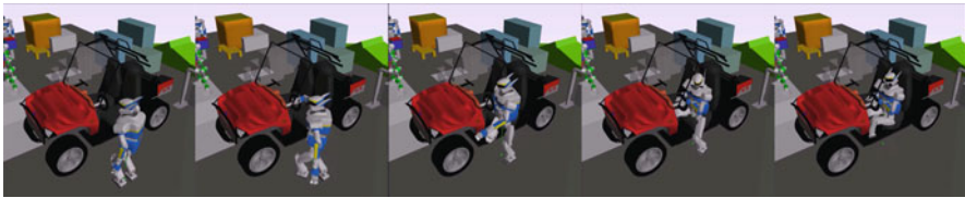
Fig. 14 Example multi-contact planning and control for a car ingress scenario
