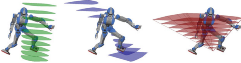
Fig. 7 Three types of support areas and volumes encoded in the contact wrench cone. Left : the right cylinder of COM positions that characterizes static equilibrium [18]. Middle : support areas for the ZMP taken in virtual planes, which can be used for multi-contact locomotion in the Linear-Pendulum Mode [25]. Right : cone of feasible COM accelerations, used for multi-contact locomotion in the Pendulum Mode [21]
