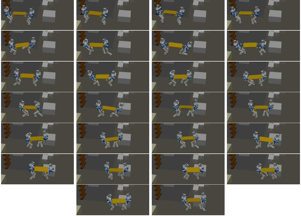
FIGURE 2.7. Collaborative manipulation. Here we use an improved version of Algorithm 2 as contacts between the hands of the robots and the handles of the table are required not to be broken during the planning, as specified at problem-instantiation-time by the user.
