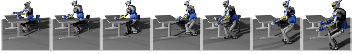
FIGURE A.4. Contacts planning for the out-of-table-and-chair scenario following the guide provided by the contacts guide planner.
